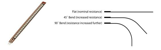
Pin P1: This pin is generally connected to the +ve terminal of the power source. Pin P2: This pin is generally connected to GND pin of the power source
