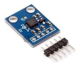
The ADXL335 accelerometer is analogue, it operates on the capacitive sensing principle. When a capacitive sensing accelerometer is moved in any direction, its capacitance changes. When the capacitance changes, the analogue voltages change, which is detected by the interface controller.
